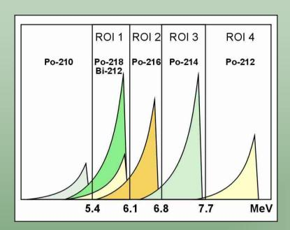
Acquisition of the alpha spectrum by a MCA connected to the detector
