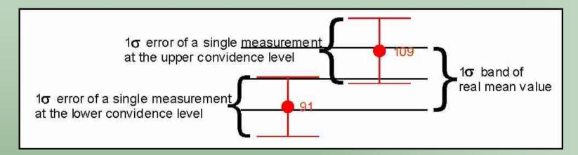
The probability that the single measurement is placed within the  $1\sigma$  band of the mean value is  $68\% \Rightarrow$  The probability that the real mean value is covered by the  $1\sigma$  error of the single measurement is also 68%!
