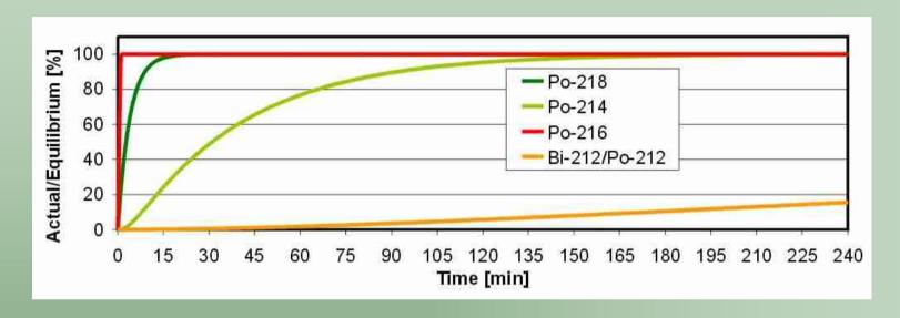
Radon calculation based either on Po-218 only (Fast Mode) or on sum of Po-218 and Po-214 (Slow Mode)
